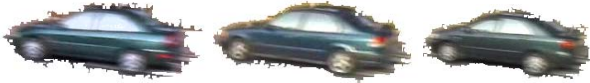
Fig. 2 : The colors of the same vehicle are different under different lighting conditions.
