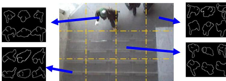
Fig. 12. Grid-based template matching for people counting; each grid uses different types of template to verify pedestrians
