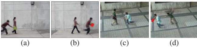
Fig. 9. Results of carried bag segmentation when the person ran very quickly. (a) and (c): Contacting. (b) and (d): Results of bag detection.
