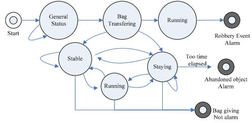
Fig. 5. Finite state machine for suspicious event detection through a bag-transferring trigger.
