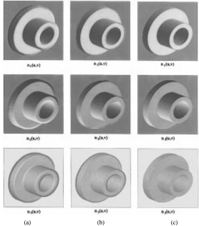
Fig. 5. Three component of normals ( $n_1, n_2, n_3$ ) estimated by using (a) quadratic surface fitting, (b) the orthogonal wavelet-based approach with three vanishing moments, and (c) the nonorthogonal wavelet-based approach.
