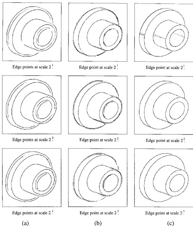
Fig. 6. Detected edge points at different scales using (a) quadratic surface fitting, (b) the orthogonal wavelet-based approach with three vanishing moments, and (c) the nonorthogonal wavelet-based approach.
