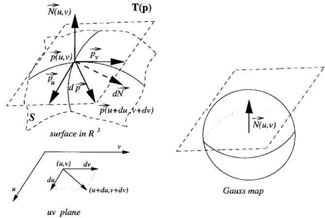
Fig. 1. Relations between a surface point, its corresponding parameter coordinate, and the Gauss map.
