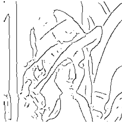
(f) Edge points from W_{2^3}^1 f(m, n) and W_{2^3}^2 f(m, n) using our method.
