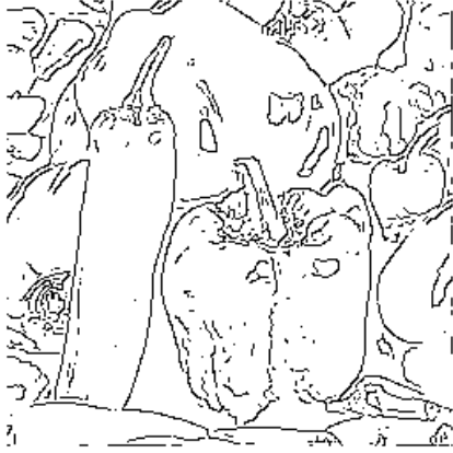
(c) Edge points from W_{2^2}^1 f(m, n) and W_{2^2}^2 f(m, n) using Mallat-Zhong's wavelet.
